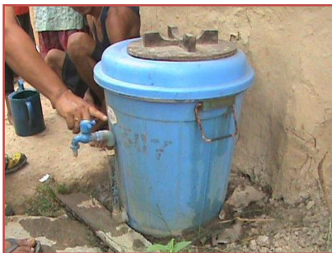
Figure 33 and 34: Plastic Kanchan ABF which is leaking and in is in use (left), a broken Plastic Kanchan filter which is not in use (right)
